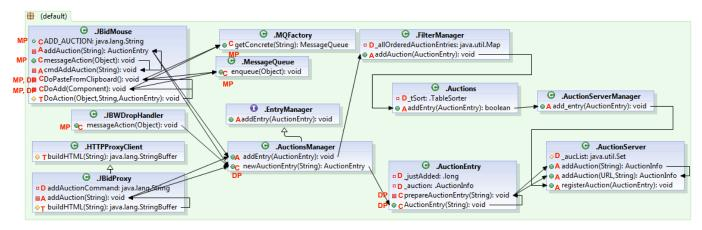
Fig. 1: Program elements and roles for the example "add new auction to local system" concern. Each element is annotated with its role in red. Edges indicate structural relationships such as calls (solid-head arrows) and inheritance (open-head arrows).
