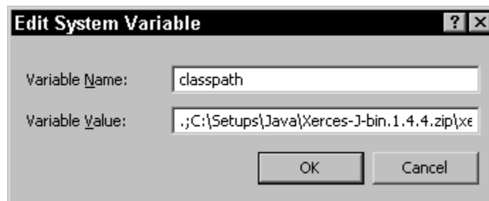
Figure 2-3: Adding the working directory to the CLASSPATH.
